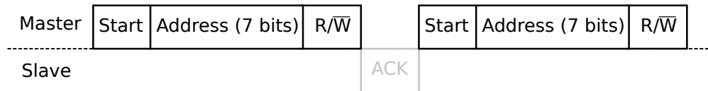
Figure 3.15: Representation of an I2C write operation without slave acknowledgement
